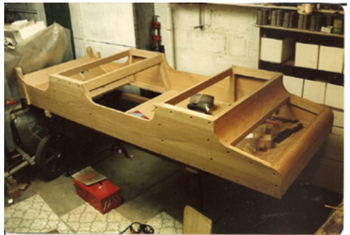
Body without seats beautifully constructed with that lovely, curved rear.
