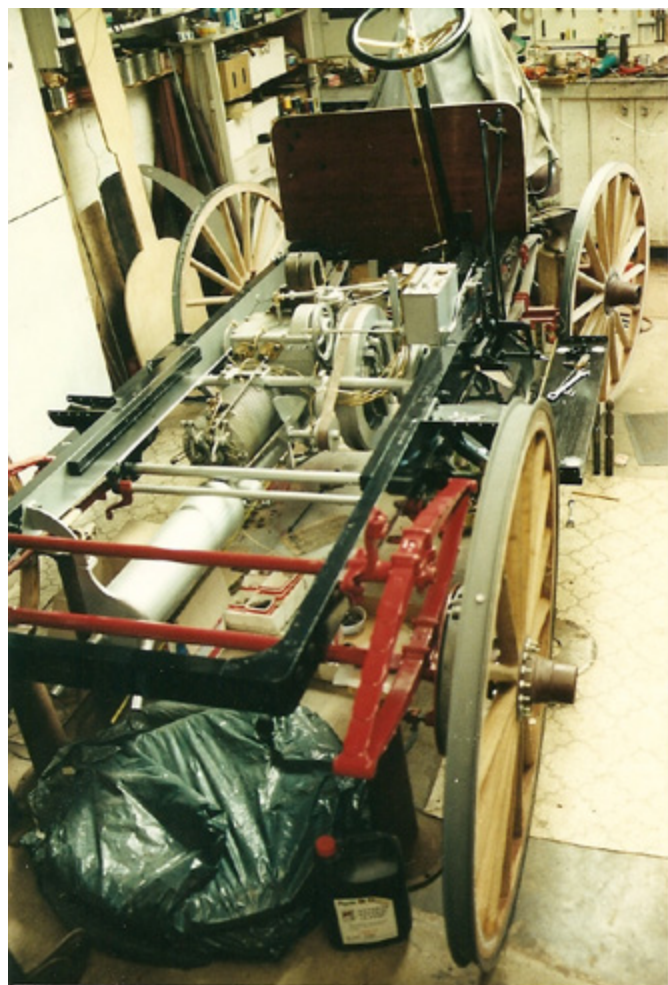
Rear view of rolling chassis, noting that the muffler has been fitted.
