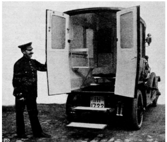
A C2K ambulance with two seats on the left-hand side, opposite the stretcher.
