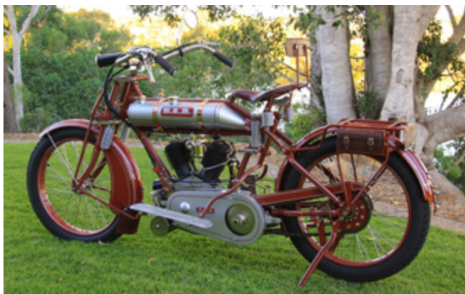
A wonderful example of a restored B&B. Note the springing from the seat to the footrest. Very unusual feature found on B&B's
