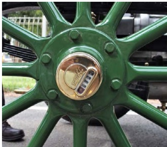
Mileage counter on the front wheel
