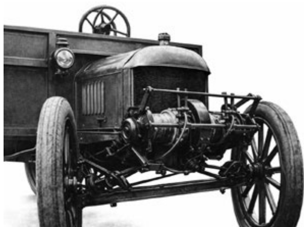
Fig 1 the front mounted winch along with the extra radius rods
