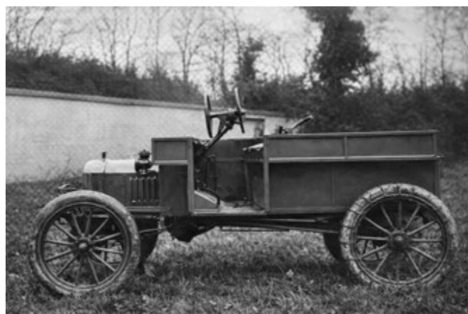
Fig 4 A side view of the Ford. Note the extra ground clearance
