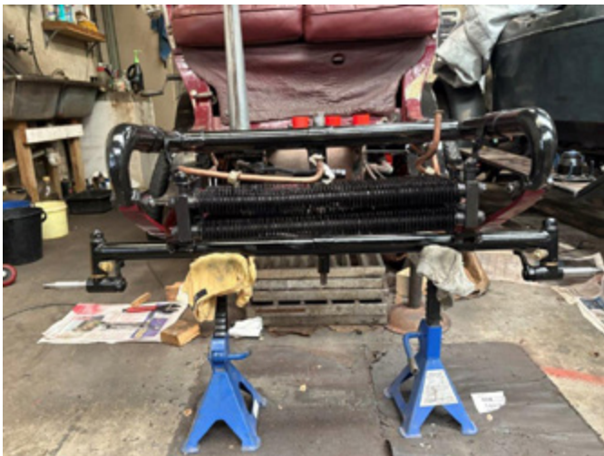
Re-tubed axle fitted, stub axles refitted from underside as previously set up incorrectly for many decades and repaired radiator fitted
