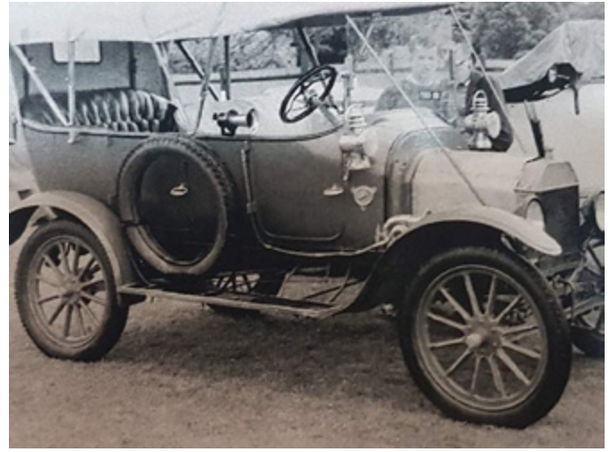
The Model T with the more modernized bonnet now changed to be back to original configuration. Note bonnet is aluminum and the side lights are still the Deitz type, also with brass horn mounted. It also now has a brass radiator
