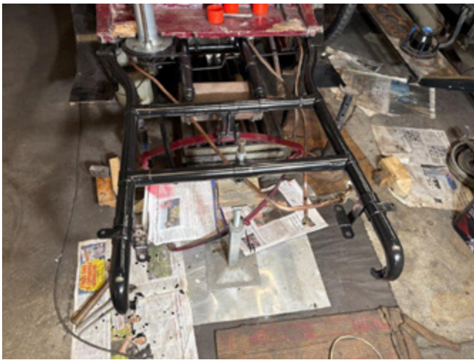
Chassis painted after the repair
