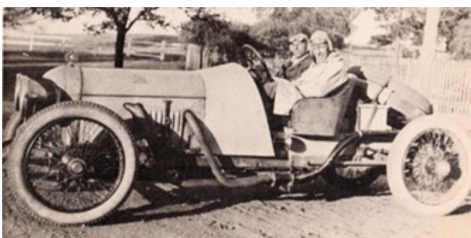
This side view at 'The Heights' confirms the unlightened brake drums and Rudge Whitworth wheels seen in 1916. (Courtesy of David Kux and Mrs Jenny Morris)
