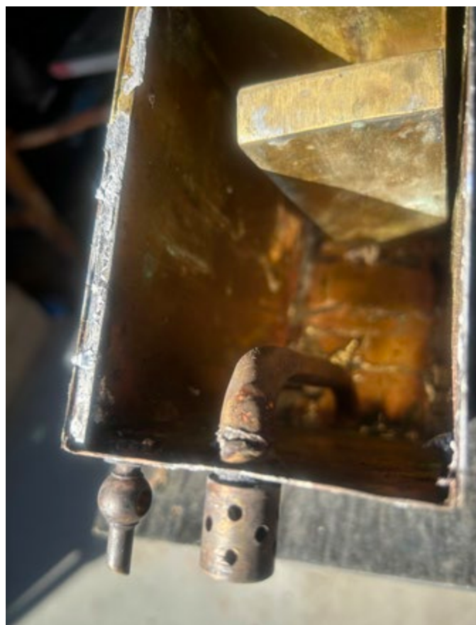
The tank apart showing the small leak around the exhaust warming pipe.
