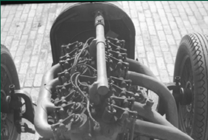
Valve mechanism of 1910 of Prince Heinrich Benz. 4 valves per cylinder
