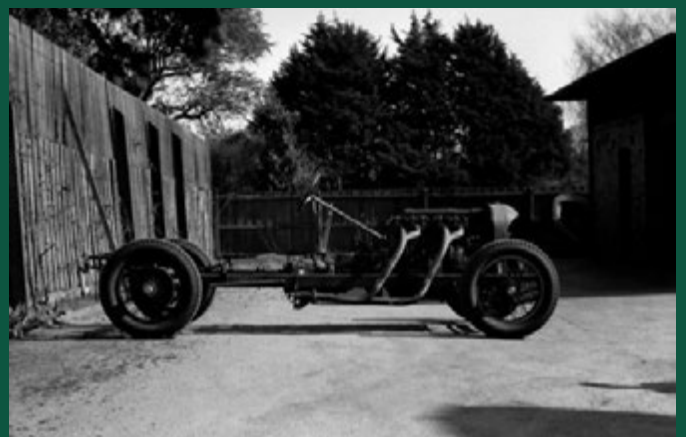
The Benz now with exhaust fitted and all wheels ready to run.
