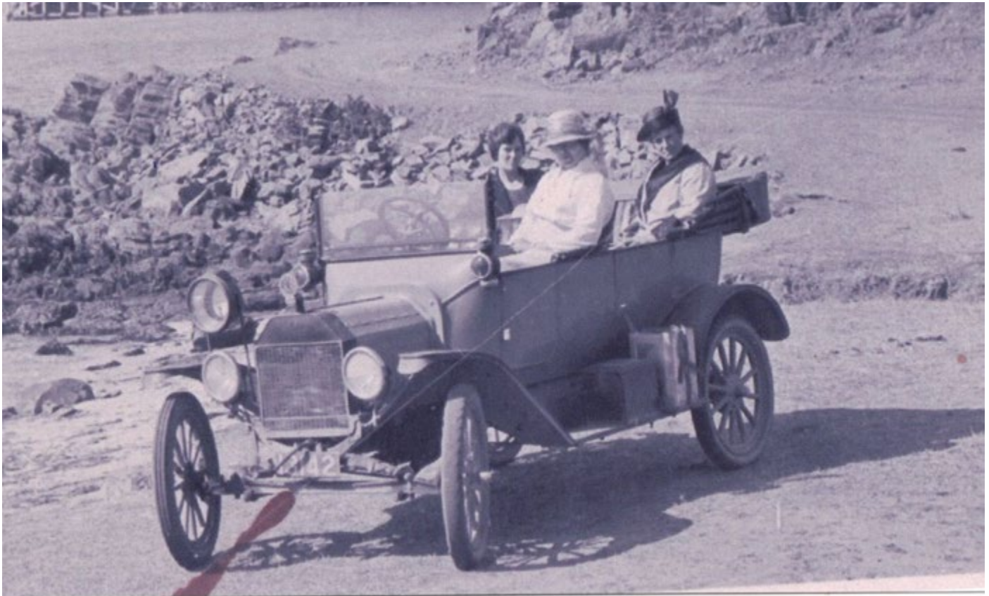
The photograph of the McAskill Ford Model T was taken very near the jetty at The Bluff, at Victor Harbor. Note the huge acetylene lamp perched above the electric headlight
