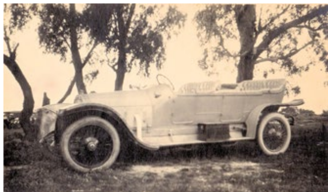
This large Benz was seen by Lou Whyte at an event in Victoria during 1914-15, possibly an 18/45, but it cannot yet be linked to Syme. It is not his 38/60. The scuttle lamps were a common Benz fitting. (Courtesy of David Kux and Mrs Jenny Morris)
