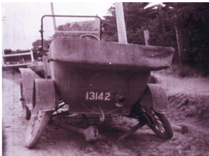
The 13142 registered Ford Model T in dire trouble with a collapsed rear end. Note the Stepney wheel carrier: this was a type that was made by Duncan and Fraser. I think it will require more than a Stepney wheel to get this one home!
