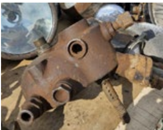
This water-cooled head was a two bolt variety, therefore not De Dion Bouton. It was likely an aftermarket item used on a tricycle or Quadricycle circa 1898-1903.
