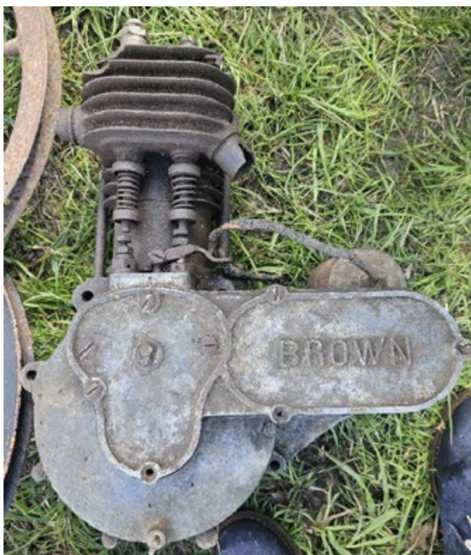
Left: This motorcycle engine by Brown (UK) looked complete but did suffer from some crankcase rot.
