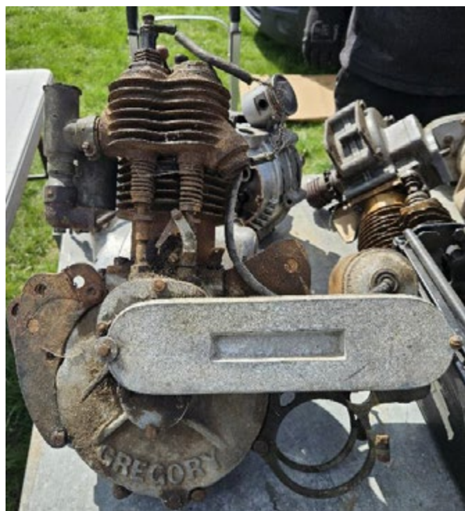
This motorcycle engine was by an obscure maker – “Gregory” was caste into the crankcase (Coventry). It was very like a similar sized JAP engine but varied in detail.
