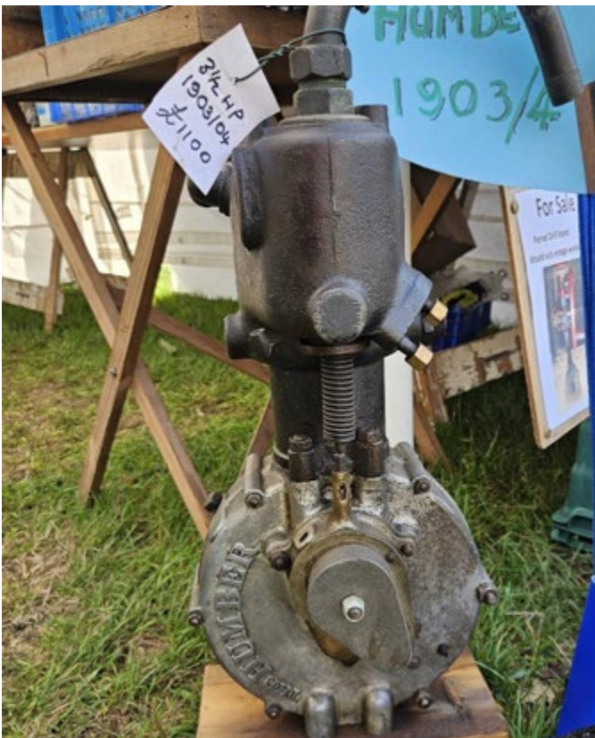
This water-cooled Humber engine dates from 1903-04 according to its owner. These would have apparently been fitted to a forecar or similar machine from that era.
