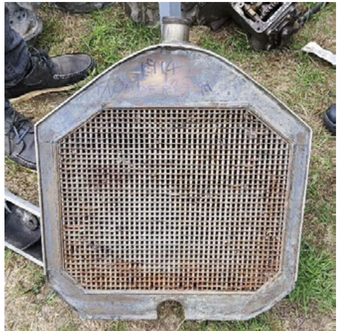
This Humberette Cyclecar radiator for a 1914 water-cooled car was a bit rough but thought to be recoverable.
