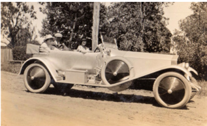
Three images of 38FW when new. He took no risks this time, lamps were fitted! Everything about this Damyon coachwork is pleasing – the neat anchorage for the windscreen pillars (with the screen's frameless glass going down to scuttle level), the straight lower hood line, the pleasant rear curves, and always of course the sporting wings. The normally exposed supplementary oil tank is here enclosed in a box next to the spare wheel.
