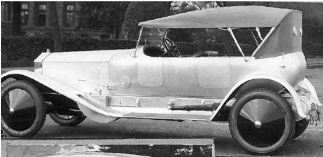
Three images of 38FW when new. He took no risks this time, lamps were fitted! Everything about this Damyon coachwork is pleasing – the neat anchorage for the windscreen pillars (with the screen's frameless glass going down to scuttle level), the straight lower hood line, the pleasant rear curves, and always of course the sporting wings. The normally exposed supplementary oil tank is here enclosed in a box next to the spare wheel.
