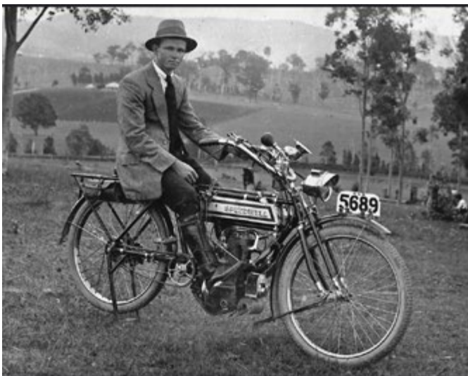
Photo above is a c1914 Speedwell FN. These were fully imported FNs carrying only the Speedwell name. Note the shaft drive.
