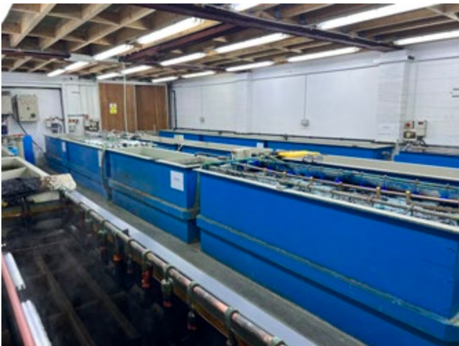
Plating baths run 4 days a week with extended hours to conserve power
