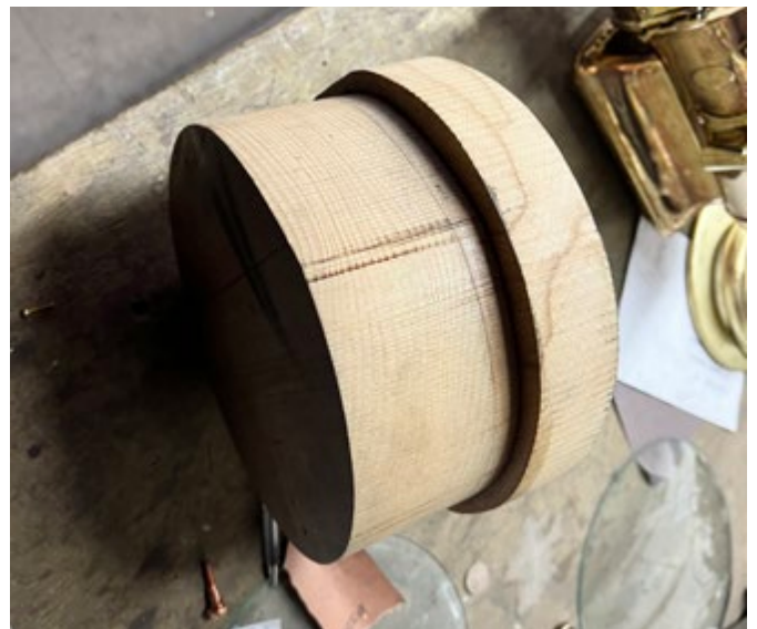
Harry's lamp rim and timber for the mould
