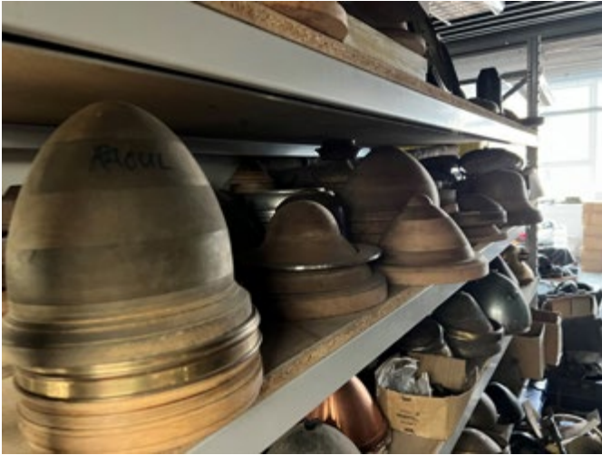
Racking of metal spinning timber moulds
