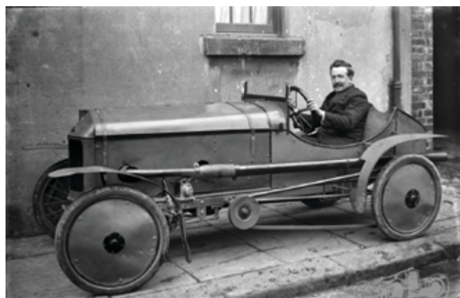
The three quarter front view shows the magneto and exhaust port locations from the front and rear cylinders of the fore and aft vee-twin engine.
