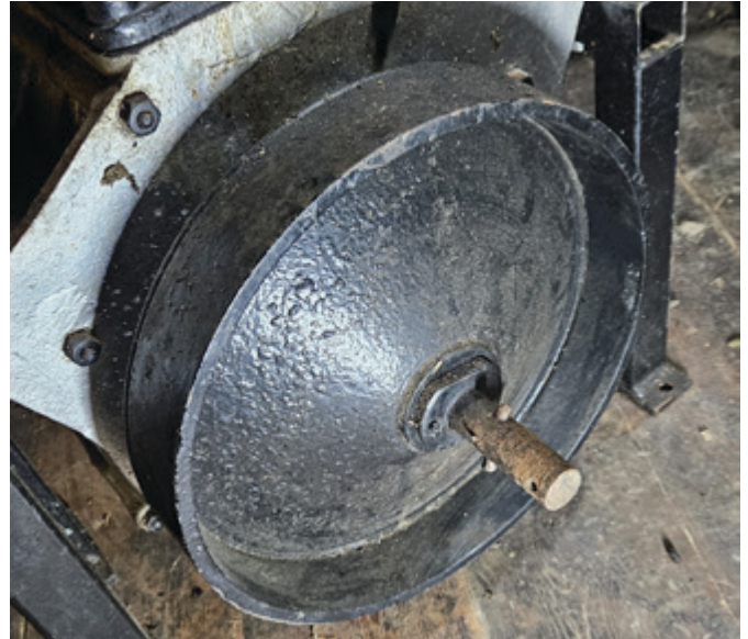
the flywheel that has the facility to receive a cone clutch.
