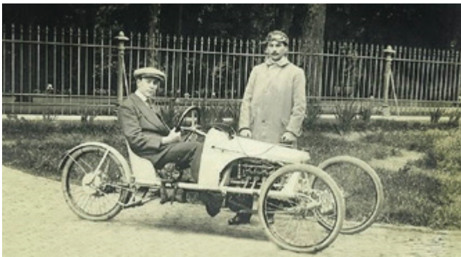
This vehicle looks to be a homemade single seater largely built using the majority of parts from a four cylinder Fabrique Nationale (F.N.) motorcycle from Belgium. Well done him! Accreditation Flickr – a European location.
