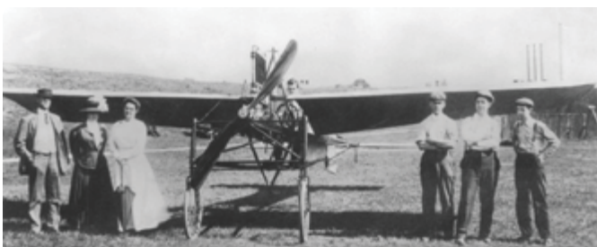
This is an example of the conversion of a T Ford engine for aero use.
