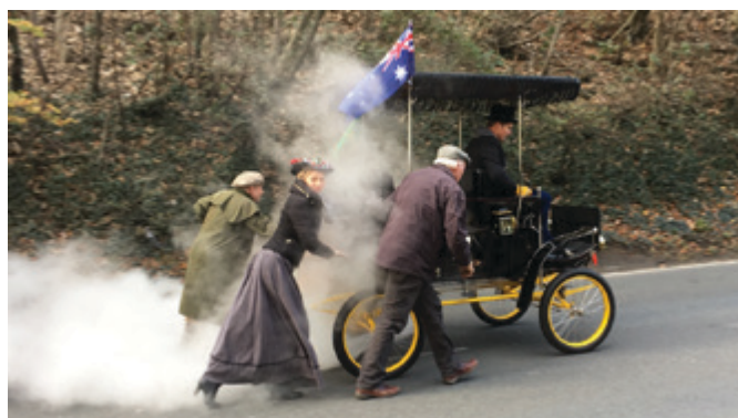
The Locomobile required a push when the boiler pressure was down on an uphill start
