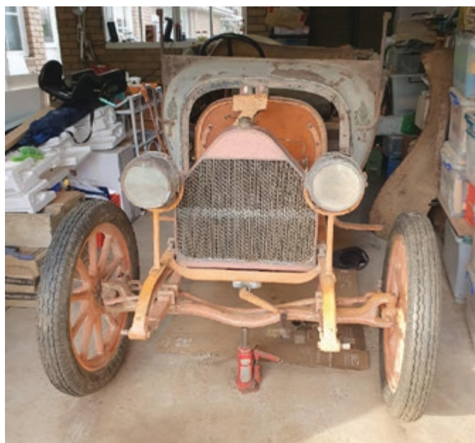
Jim's fabricated radiator, to the same size and shape of the original.
