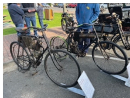
Left is the c1902 De Dion powered bicycle with a surface Carburetor
