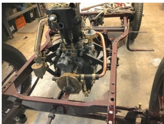
The newly restored 150mm long stroke CP De Dion engine with mechanical valves installed
