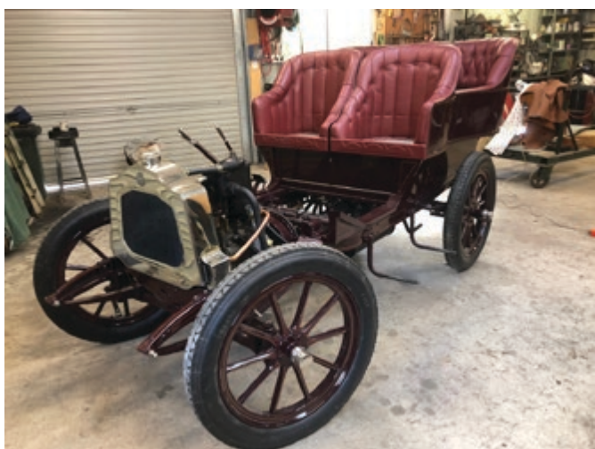
The body back in place on the rolling chassis
