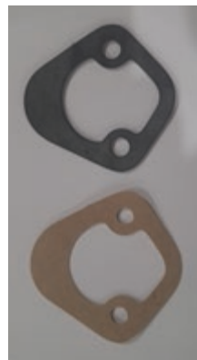
Original gasket (top) Reproduction from scanned image (below)
