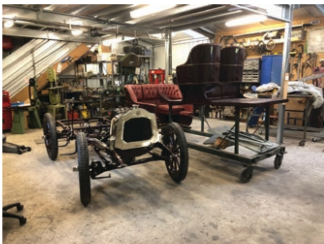
Chassis ready to take the newly painted body. The radiator is all freshly plated.
