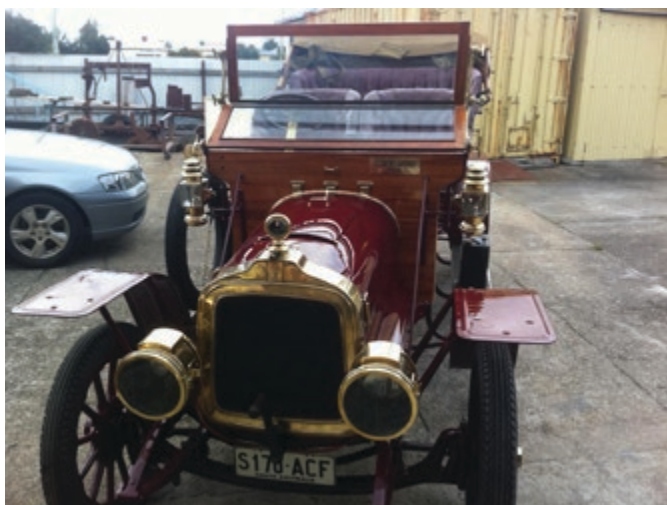
My 1908 Bayard (despite what it states on the brass plate on the dashboard) showing the three bonnet hinges and lack of bolt in the radiator
