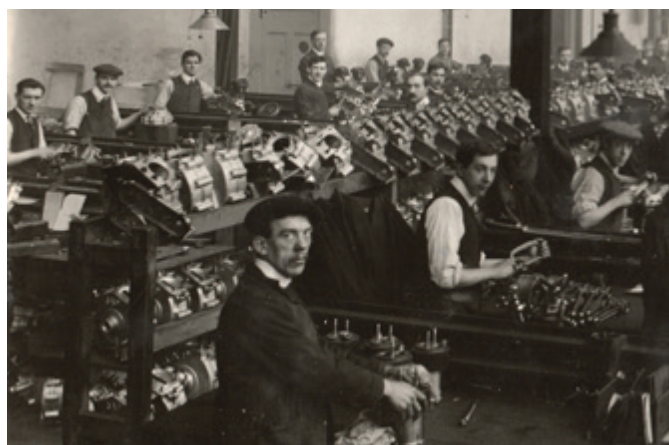
This is the JAP factory parts hand finishing area– circa 1912-13. This was quite a vast area with only a small part shown here. Interestingly the workman in the foreground is assembling the overhead valve engine version – perhaps a 90mm bore.
