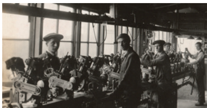
This is one of the JAP factory engine final assembly and possibly testing areas – circa 1912-13. Again it is particularly interesting because it shows both 1912 and 1913 engines being assembled side by side. There are a number of Cyclecar engines clearly visible – apart from the motorcycle type. In particular, the water-cooled item (third from left) and the special 90 degree engine further along (note the overhead inlet valve to each cylinder).
