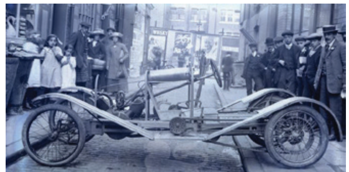
The DUO Cyclecar with 90 degree, 9hp JAP engine of 1096cc. (photo credit Stilltime, UK).
