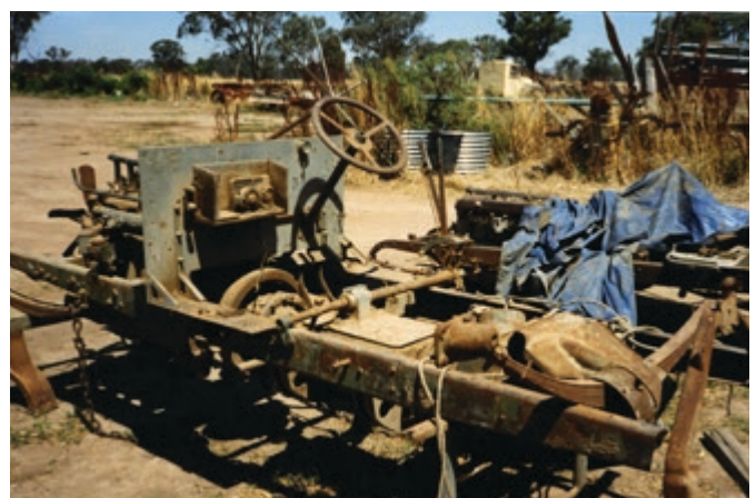
The sad remains of the Napier at Arthur Lang's property. The "home made" rear chassis member can be seen where the chassis has been cut.
