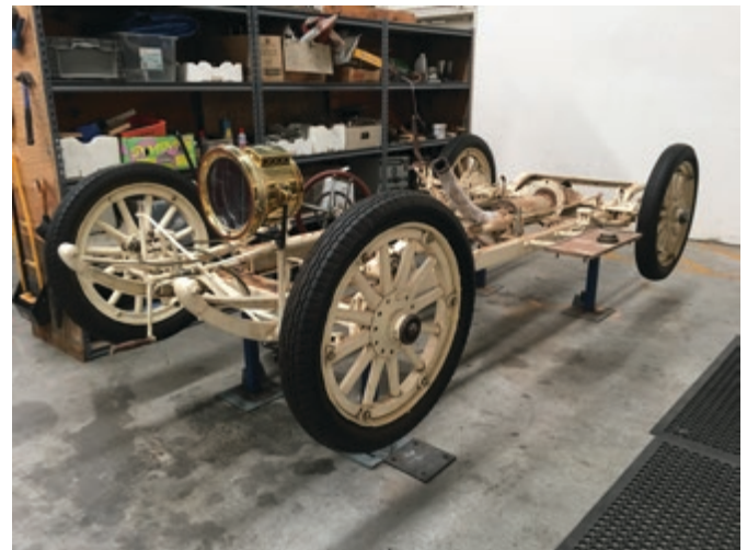
Andrew Benoit's Regal underslung chassis in the process of restoration
