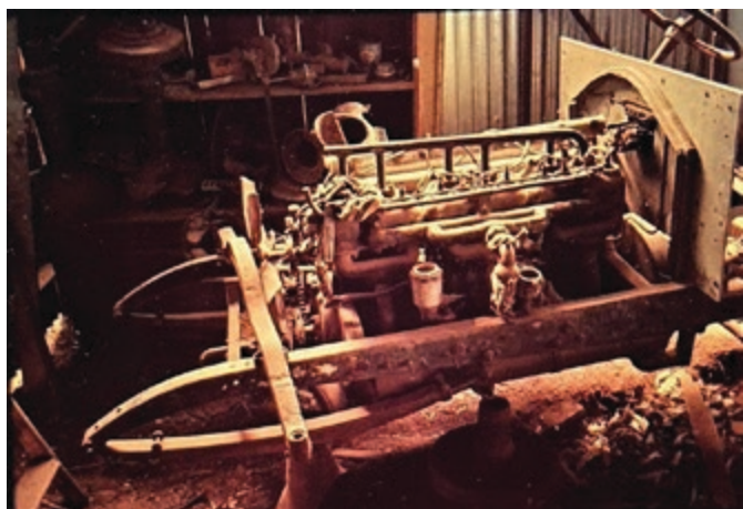
The "mystery" 6 cylinder Napier engine photographs taken in the 70s. Note two water pipes per cylinder
