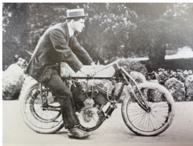
One of several motorbikes built and raced by Harry and his mates, Harry Busteed and Cecil de Fraga. The rider had to sit over the rear wheel and use long handlebars because the engine was so large.
