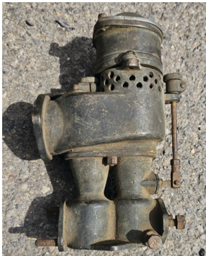
Above, the twin jet RR 40/50 carburettor found at the Bendigo swap meet.
