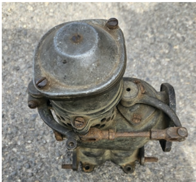
This is the top of the 40/50 twin jet carburettor offered up at Bendigo.
