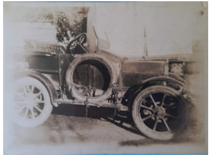
Part of the modernisation that occurred c1920 of the body and mudguards. Note the now rounded mudguards
