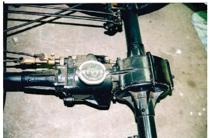
Figure 6. The Type A Stutz transaxle fitted to the Empire 20. Note the two independent brake control levers at the top of the picture.
