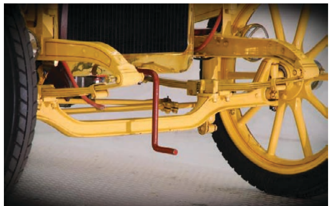
Figure 10. The Empire Model C front axle shackle mount.
