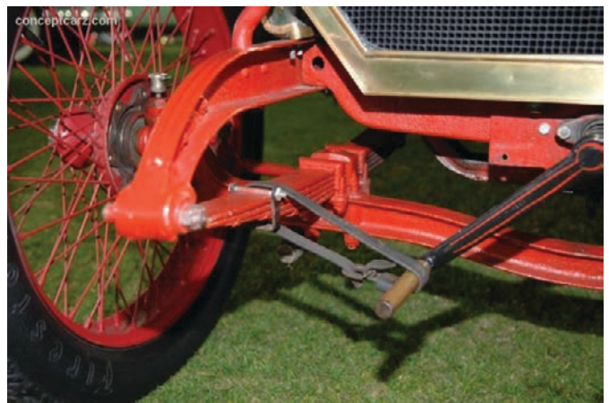
Figure 9. The Marion 10 front axle shackle mount.
