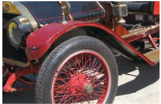
Figure 13. The Marion Bobcat showing front fender with characteristic drooping eyelid.
