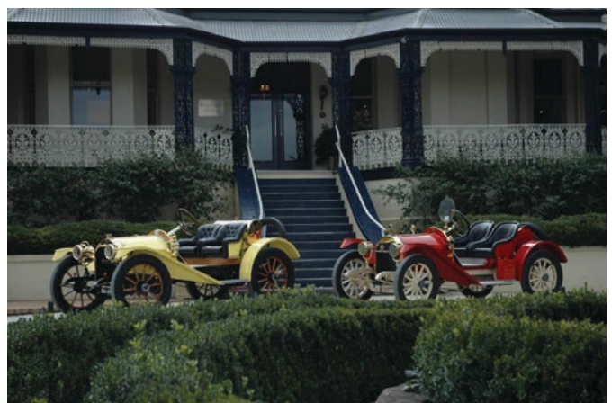
Figure 12. The two Empire-20 Model C survivors in Australia showing drooping eyelids on front fender.
