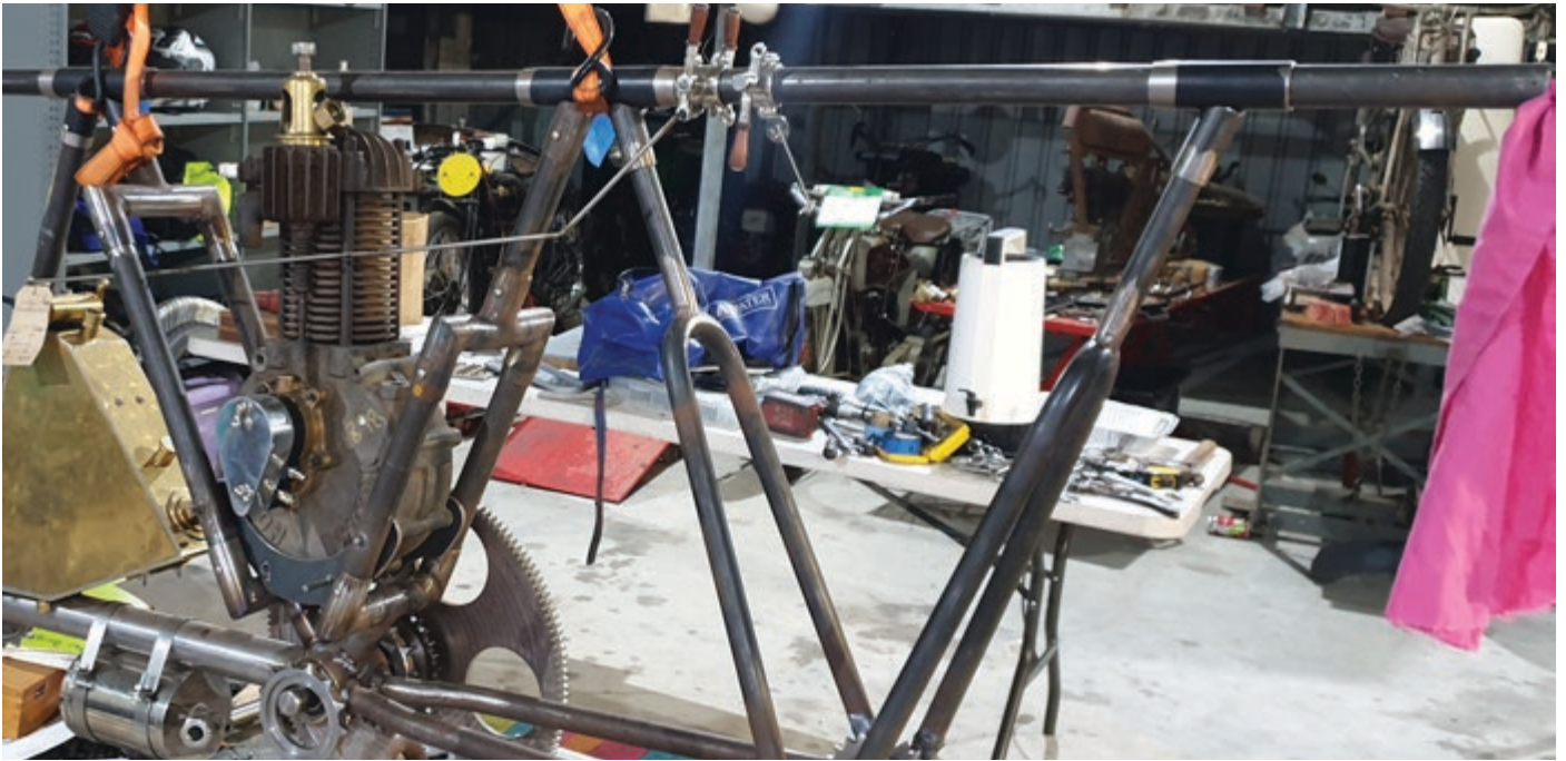
This is the frame and components that have been roughly assembled to show the huge amount of work that has been done to get this De Dion powered tandem back on the road.
