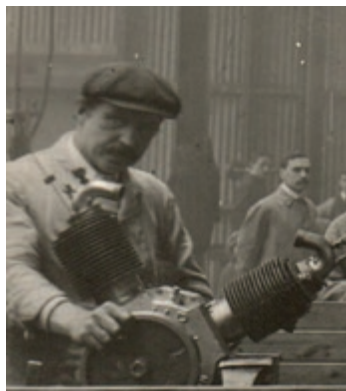
This first shot shows an engine assembler fitting up an engine – the new style 1913 type.
