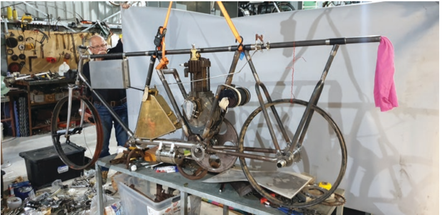
This is the frame and components that have been roughly assembled to show the huge amount of work that has been done to get this De Dion powered tandem back on the road.
