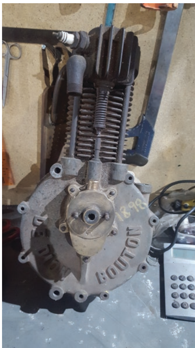
The surviving De Dion Bouton engine from the tandem.
