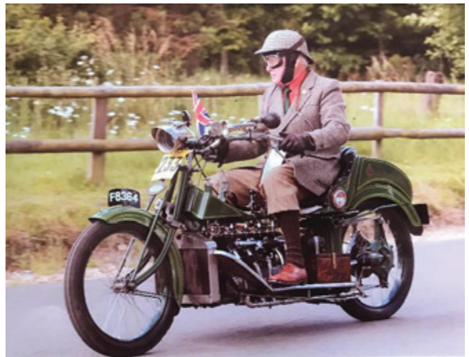
Above, a Wilkinson motorcycle survivor in the UK. The radiator on this machine looks to be identical to that used in their car – apart from the differing brackets and lack of apron.
