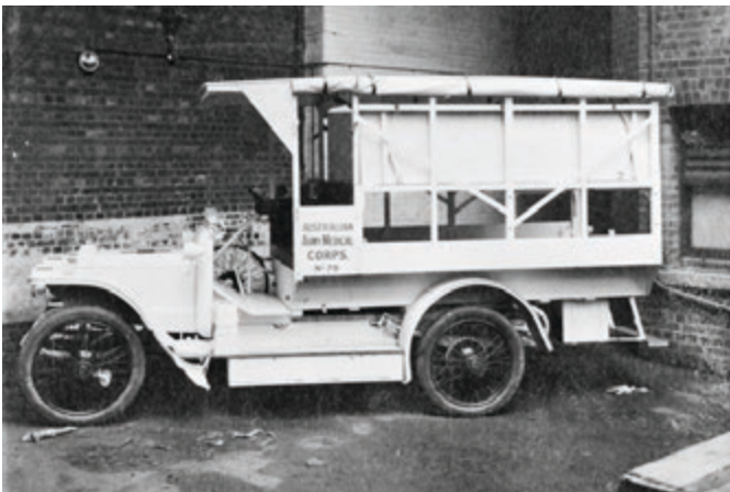
A 1910 15 h.p. Daimler ambulance of the Australian Army Medical Corps with possibly a body built in Australia. [Australian War Memorial PO2869.003]
