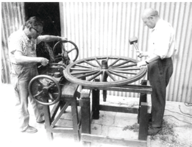
Laurie Vinall and Ron Sambell fitting a tyre using the Dunlop horizontal tyre machine
