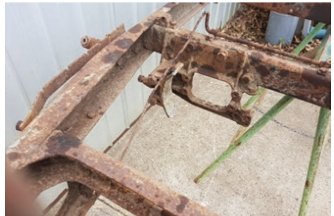
Above, the area under the seat showing the transmission brake (part complete).
