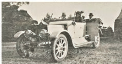
The year of this one is more likely 1913, with electric lighting and Stanley steel wheels. The family is said to be Road, at Mt Lady. With no registration number, the owner can't be confirmed, but the location can, with the base of the steeple in the background. The length of the bonnet suggests a six cylinder motor, a number of which were on the road in SA.
