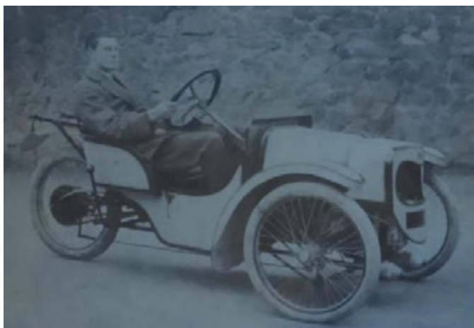
Above, this is a Standard Model of 1912 – the external gear lever is just visible behind the hand brake. This car is the base model - no extras present.
