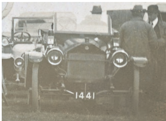
A very nice 22hp Metz which was a successful friction drive vehicle.
