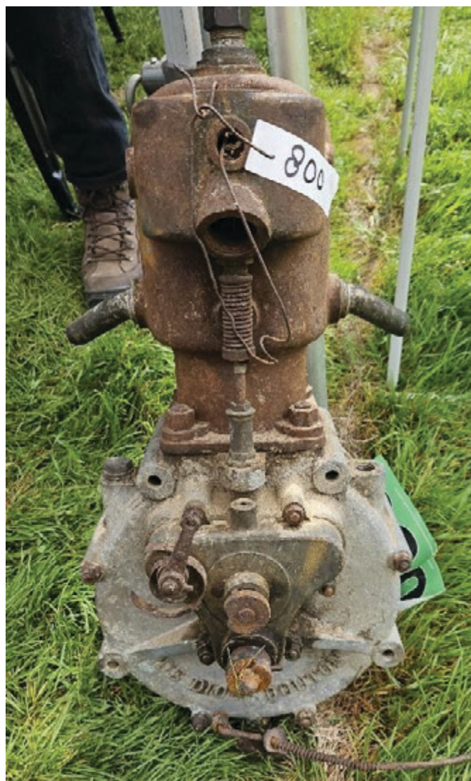
Above, an early single cylinder De Dion Bouton engine. It looked to be 4.5hp
