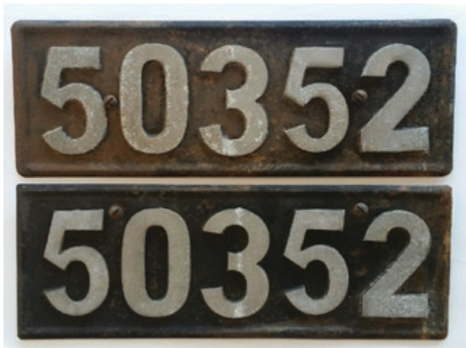
Above: These Victorian number plates were made commercially largely in the 1920s. They were made of aluminium – numbers riveted on.
