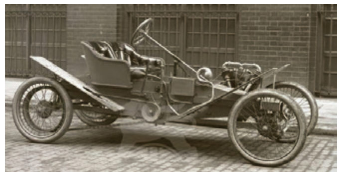
A creditable concoction – JAP engine and Chater Lea axles and wheels. (Accreditation, Stilltime UK). Interestingly the engine has atmospheric inlet valves. This is rather unusual for a vehicle this late. However JAP did catalogue these as late as 1912 (approximately).
