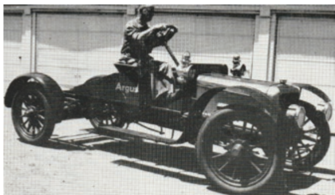
Part-restored chassis with temporary seat. Original wheels with new rims and 880 x 120's. Copper radiator shell.
