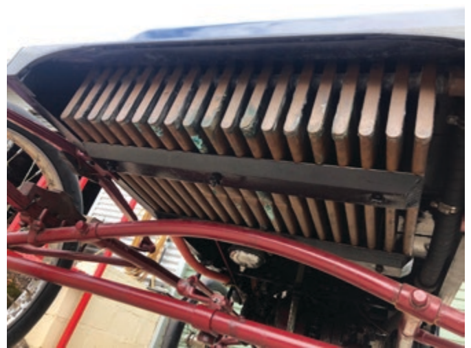
Radiator situated beneath the front floor
