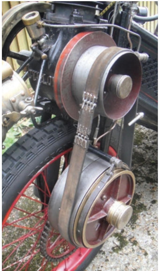
Cyklon drive set up with the flat belt.
