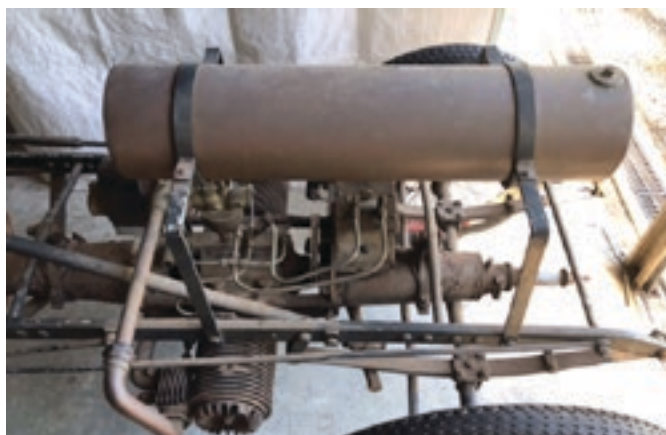
The engine is a Holsman and would have come from a motor buggy – prior to 1911. Refer photo.
