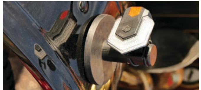
Bicycle indicator attached to a nylon rod & screwed onto the studs in the magnetic pads
