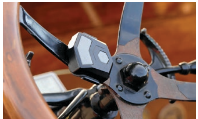
Wireless remote control switch for the indicators and hazard function mounted on the steering wheel
