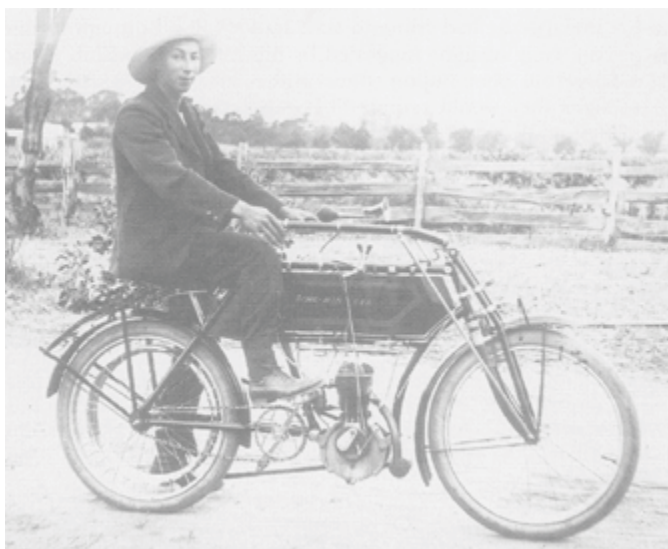
A proud William Ying on his Acme-Minerva c1906. This motorcycle was built by the Acme Motor and Engineering Co. in Melbourne, and is fitted with a 2 3/4hp Minerva engine.
