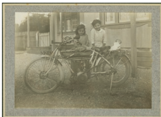
Nancy and Dorothea with their father's motorcycle photographed c.1920. With a Chater-Lea frame, Druid forks and a Peugeot engine, it is extremely likely to be of Australian assembly c. 1913-15.
