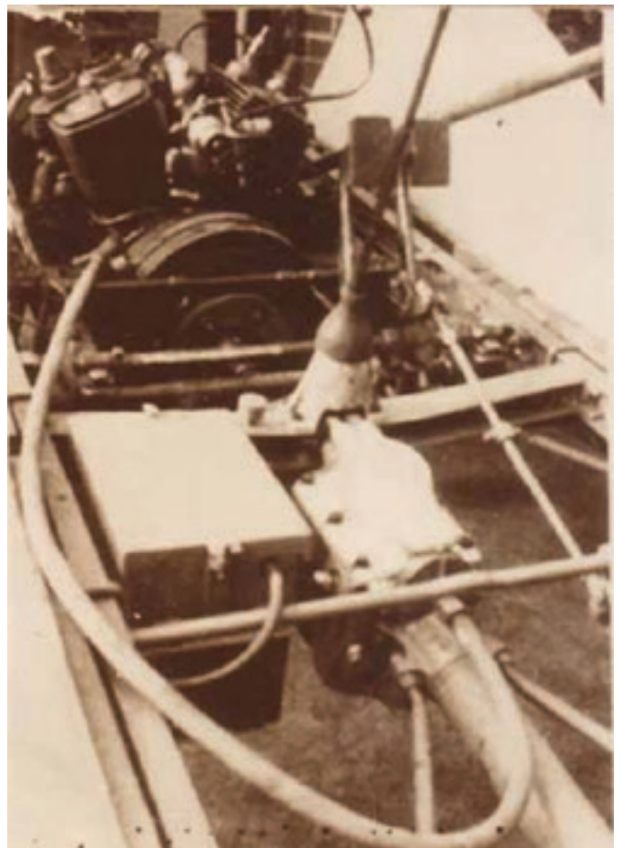
Chassis detail of the vehicle – clearly showing the Precision vee-twin engine and Barney's drive-train.
