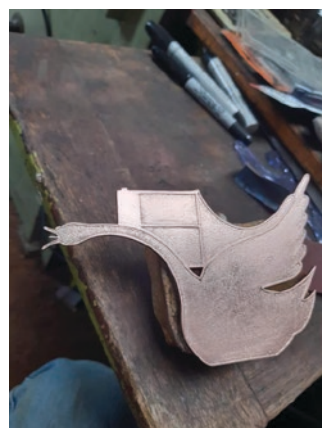
Before: Copper shape with hand drawn masking pen. After: etched.
