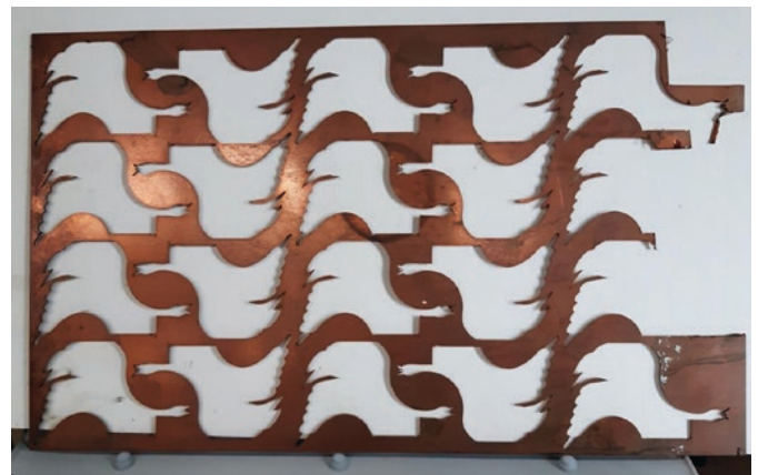
Waste copper after laser cutting the shapes.
