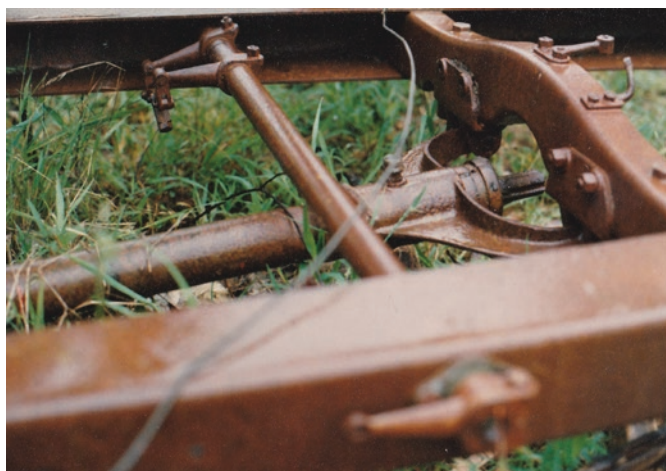
RAPID chassis – central section showing the torque tube and cross-shaft.
