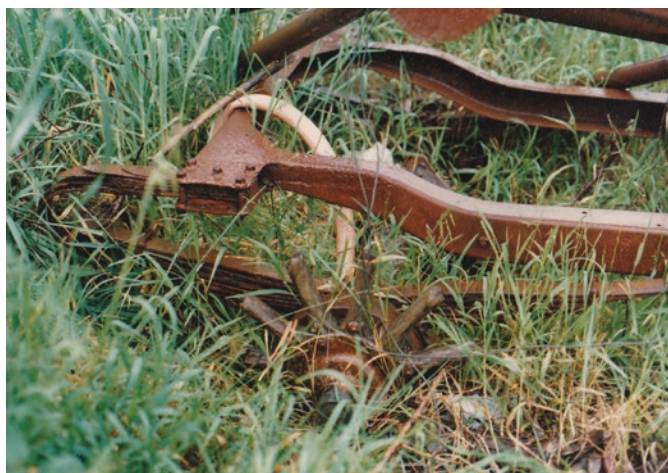
RAPID chassis – from the rear corner showing rear axle and springs
