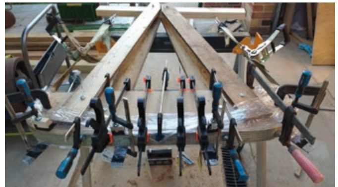
Glued up, wrapped up and clamped up
