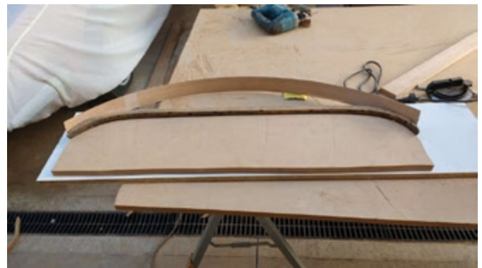
The piece to be made, the former template and a single laminate
