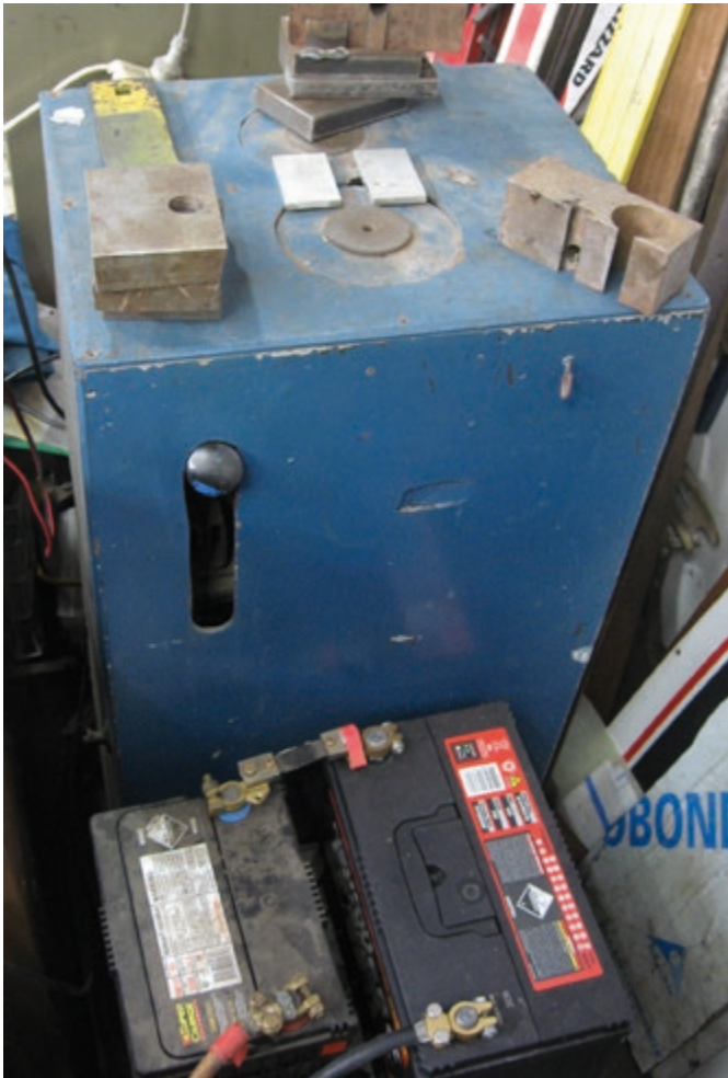
The piece of equipment is a magnet re-magnetiser. It looks weird and makes strange noises but does the job.
