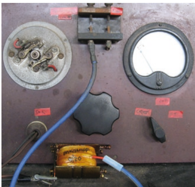
A newly wound and varnished coil undergoing an operational test prior to refitting to the armature spindle shafts. Note the small spark (light blue) jumping across the test gap near the top of the photo.
