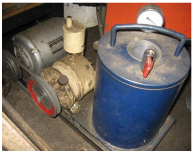
This is a partial vacuum chamber. It is used to assist in the sealing of the newly rewound coil. The process involves fully dipping the new coil into varnish then placing it into the partial vacuum tank – where most air is removed to allow varnish into all voids. The coil is then baked in a oven to properly set the varnish. Excess varnish is then removed from the outer steel bobbin areas.
