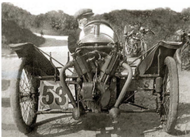
This early Morgan single seater is fitted with the 90mm bore JAP engine. These were a higher performance engine in light of the overhead valves. They were used in the early Grand Prix cars and enjoyed many successes.
