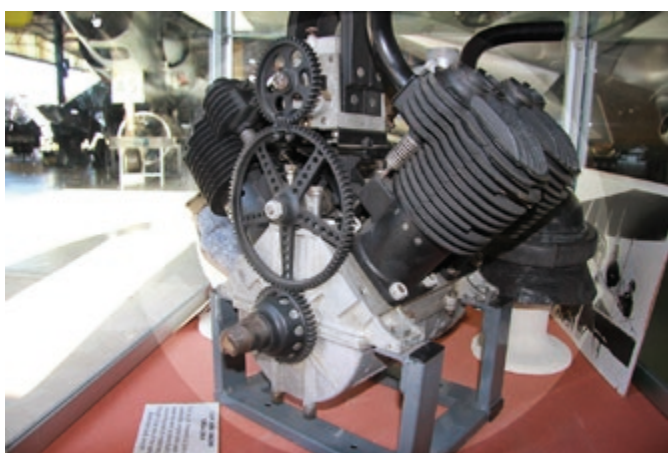
This JAP engine was designed for use in an aeroplane. It is a vee-four configuration – cylinders at 90 degrees. The Australian National Aviation Museum at Moorabbin has this engine on display.
