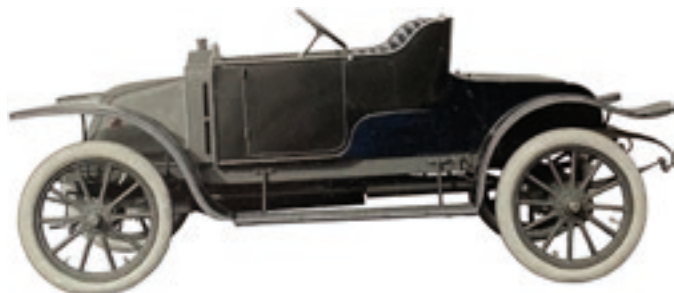
A Munro bodied single seater 1911 Clement-Bayard incorporating the new tapered-front style.
