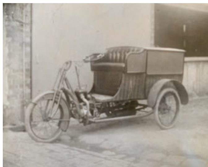
A Wall Tricar from 1913. Munro had this agency for a very short time as, by then, three-wheelers were somewhat obsolete. The Tricar was powered by a Precision motorcycle engine mounted on a tubular frame. An oval 'steering wheel' incorporated the carburettor and spark controls although steering was by tiller mechanism.
