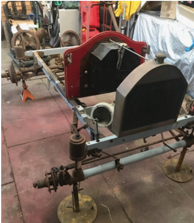
Brush partly assembled to gauge what is missing.
