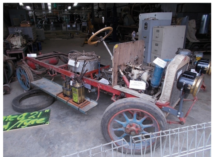
c1908 White Steam car being restored by the by Warwick Bryce and helpers at the Melbourne Steam Traction Engine Club.
