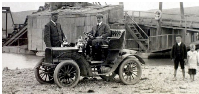
A French bodied 6 h.p. Type 2 Lacoste built Etoile with the customary back seat detached.
