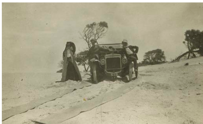
The Daimler stuck on a sand hill near Woods Wells as reported in Victorian Leaders in the Motor Car World . Wagstaff took two pieces of matting each of 36 feet length and 16 inches width. They used them on seven occasions to overcome the challenges of driving through deep sand. (VCCA)
